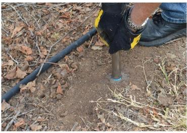
Gently, take off the **metal insertion** after installing the probe.
