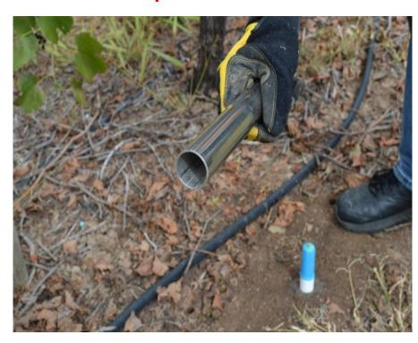
By using **a metal insertion**, you can push the probe accurately down. (use vertical position)
